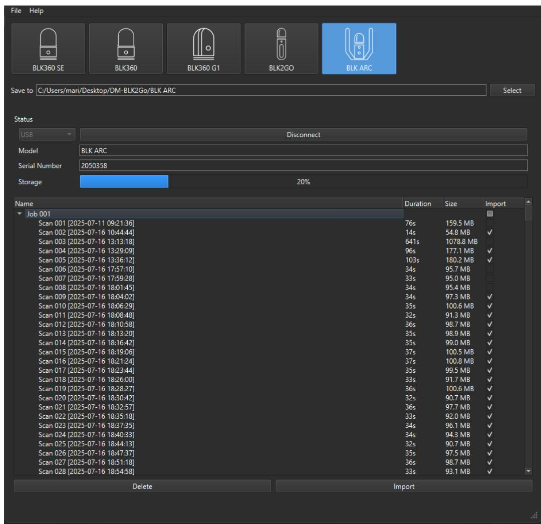
The PinPoint BLK Transfer Tool can connect and download scans. By default, all the scans are checked to be imported. In addition, BLK Transfer Tool keeps
