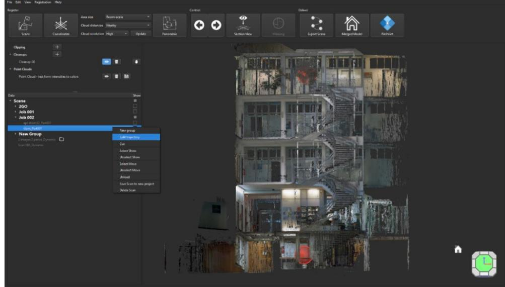
The split is possible by moving the small red sphere along the trajectory colored by timestamp.
